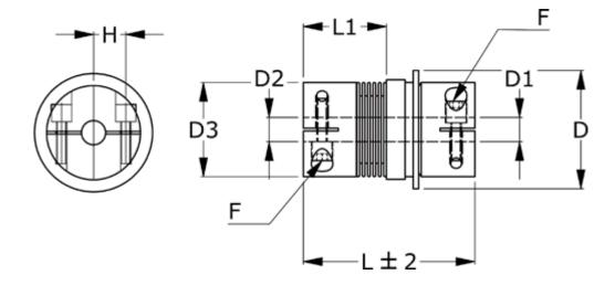
D = 109 Nom. torque NM (Tkn) = 90NM overload torque range 1 D1 = 38 Position engagement = C = Synchronous
